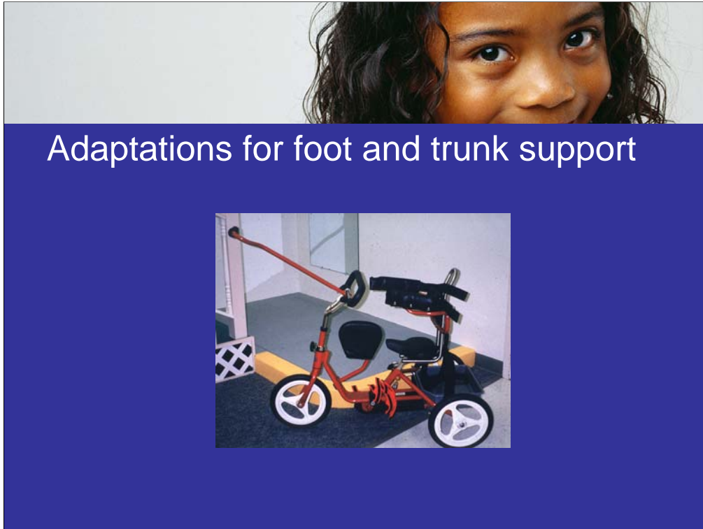
This bike has a pull stick which is used to teach a child how to ride a bike. (Rifton)
